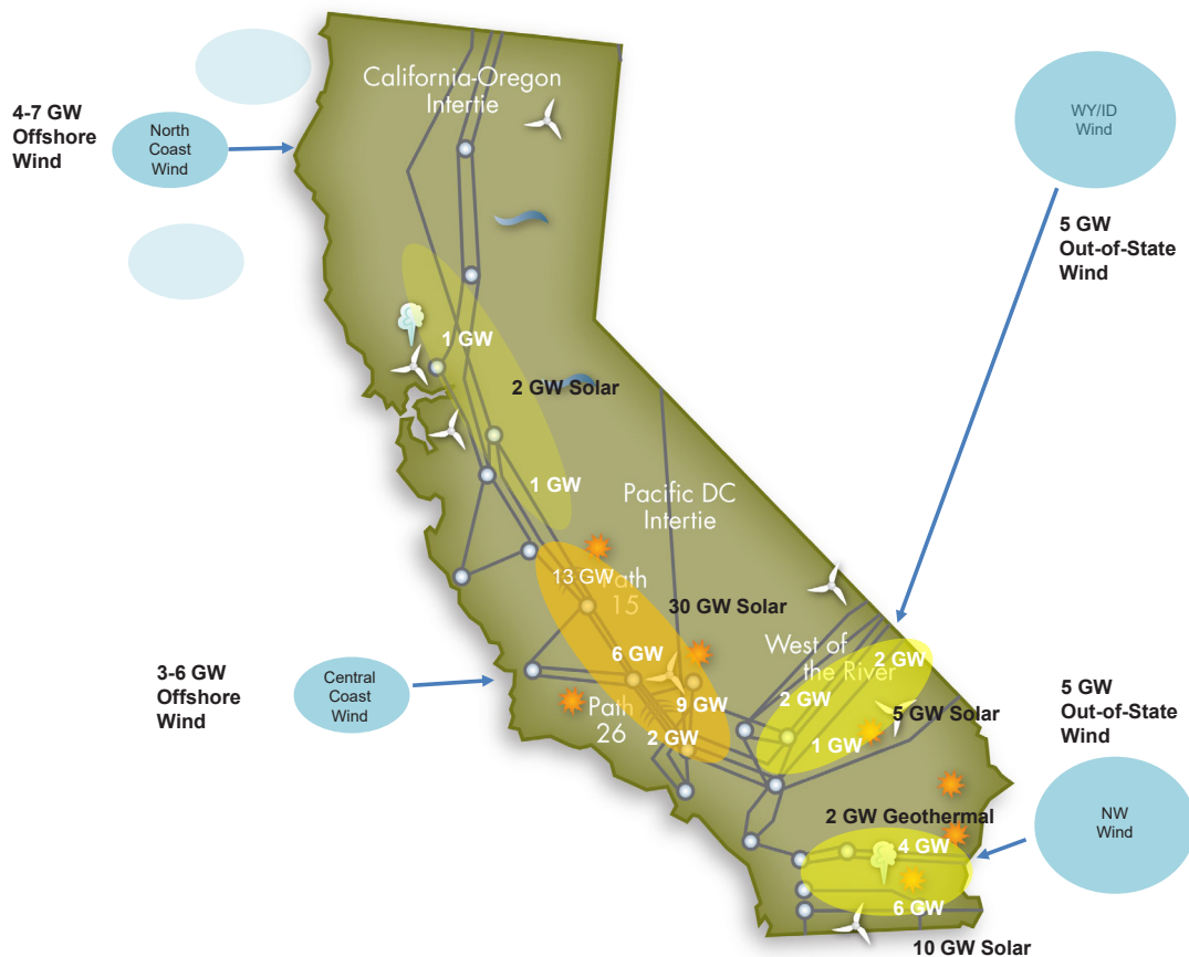
Figure 6.1. Illustrative map of candidate points of interconnection to integrate offshore wind resources to meet SB 100 high electrification load projection by 2040. 42
